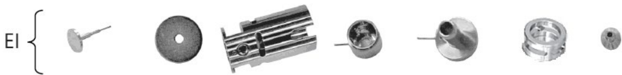
Figure 3. EI ion source parts to clean
