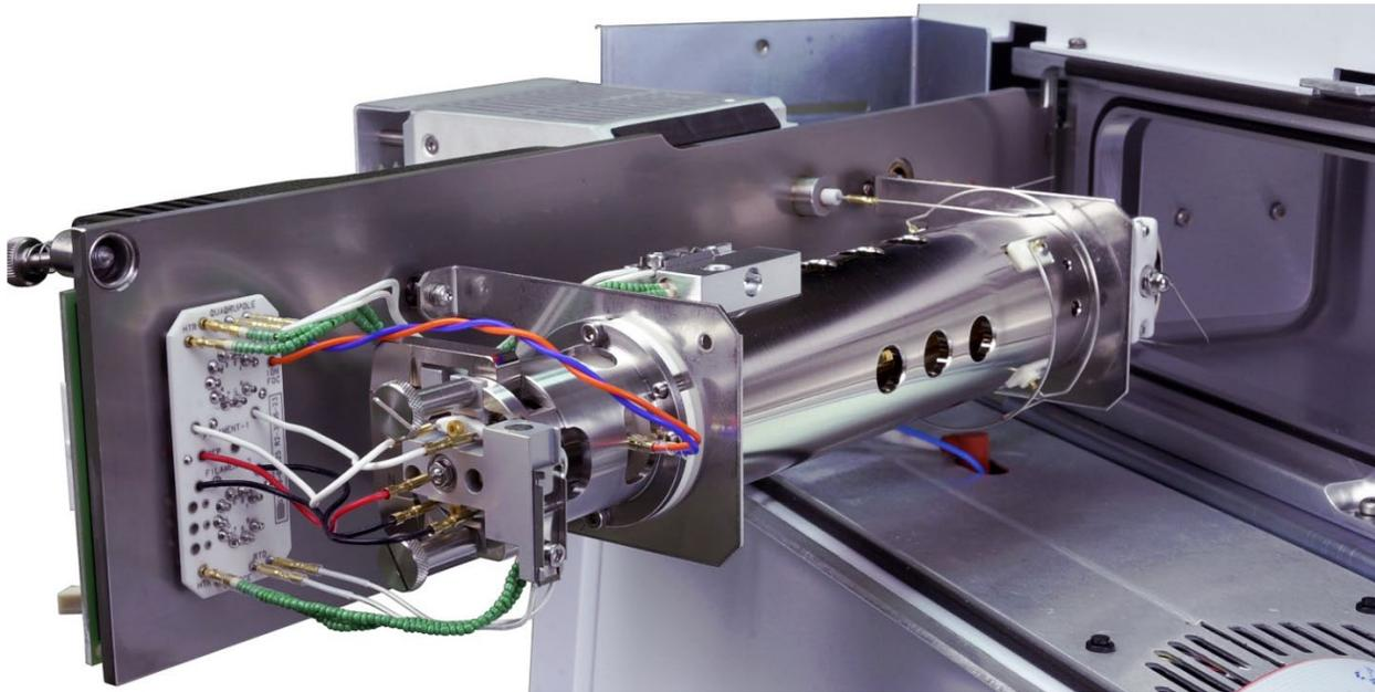
**Figure 2. EI ion source in open vacuum manifold**
